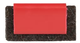
For use on M.I.G. wire feeders to remove dust and dirt from wire prior to wire entry into the liner conduit. Use of Wire Feed Pads can decrease the coefficient of friction in the liner as much as 50%. Reduces erratic feed and burn back. For use on steel, stainless steel, hard facing silicon bronze, solid and flux core wire. Treated pads may be re-treated with Wire Feed Pad Lubricant (Product No.
