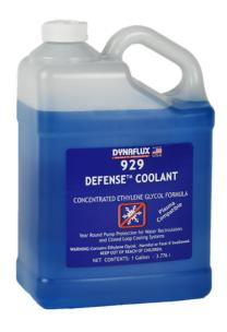
929 provide year-round pump protection for water recirculators and closed loop cooling systems. Reduces the need for water fill maintenance by reducing water evaporation. The concentrated 929 formula protects from freezing to -30°F when not diluted. A dilution of 2 parts Defense 929 to one part water will protect to -10°F.
