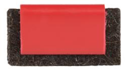
For use on M.I.G. wire feeders to remove dust and dirt from wire prior to wire entry into the liner conduit. Use of Wire Feed Pads can decrease the coefficient of friction in the liner as much as 50%. Reduces erratic feed and burn back. For use on steel, stainless steel, hard facing silicon bronze, solid and flux core wire. Treated pads may be re-treated with Wire Feed Pad Lubricant (Product No. 502).
