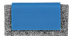
For use on M.I.G. wire feeders to remove dust and dirt from wire prior to wire entry into the liner conduit. Use of Wire Feed Pads can decrease the coefficient of friction in the liner as much as 50%. Reduces erratic feed and burn back. For use on aluminum wire when welding on aluminum.
